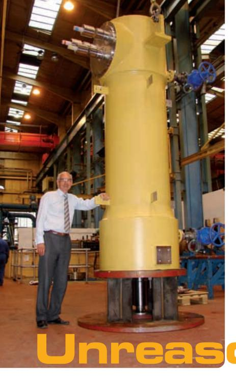
motor of vertical shaft design, weighing in at 12.5 tonnes and measuring 3.3 metres from top to bottom, capable of running at up to 4,000rpm.
